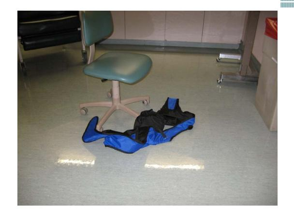
Here is another picture of how **not** to care for the aprons. When aprons are not properly handled, they crack and damages the lead.
